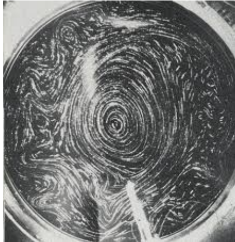
Figure 9: A rotating dishpan experiment of the type normally conducted by Dave Fultz and his colleagues in the 1950's (and now common all over the world). The thermal difference between the heated edges and the cooled center of the dishpan creates motions, which by the rotation develop wave motions very similar to the atmospheric flow at jet stream height 9-12 km.
