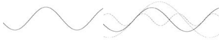
Figure 1. A CAV-trajectory (above) and (below) the corresponding progressive, short wave length streamlines (long dashed lines) and the retrogressive, long wave-length streamlines (short dashed lines) it satisfies.
