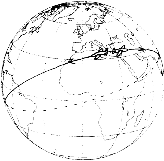
Fig. 1 The deviation of an aeroplane initially moving along a latitude, following a great circle, has nothing to do with the Coriolis effect since the deviation is always to the south in the Northern Hemisphere for westward and for eastward motion
